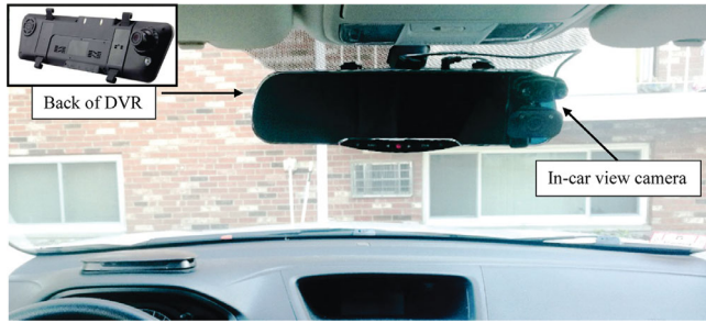
Figure 2. Digital Video Recording (DVR) system built as a rear view mirror. It is comprised of a front-scene view camera, a small in-car view camera on the far right side of the mirror, and a GPS recording device. The camera system did not impede participants' view through either the windshield or mirrors.
