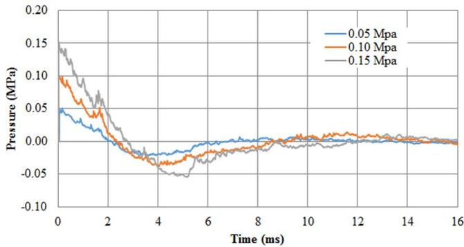
**Figure 3.** Overpressure-time histories from physical experiments using the shock tube.<sup>17</sup> These were selected as representative for three levels of blast and applied as a boundary condition in the present model. Legend entries correspond to the peak overpressure for each waveform.
