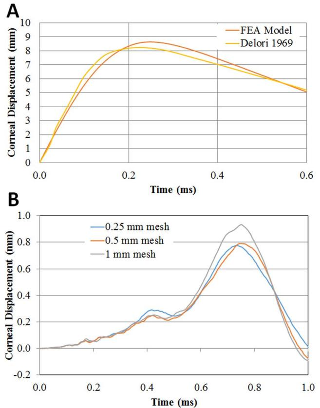
**Figure 4.** (A) Corneal displacement-time history for simulation of BB impact compared to the data of Delori. (B) Corneal displacement-time history for simulation of blast exposure for the three characteristic mesh sizes. Increasing mesh density beyond a characteristic element length scale of 0.5 mm did not significantly alter the time course of the predicted deformations.
