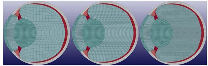
**Figure 2.** Cross-sectional view through the optical axis of the modeled porcine eye. The assembled eye model was meshed with three different characteristic hexahedral element length scales: 1 mm (left), 0.5 mm (center), and 0.25 mm (right).
