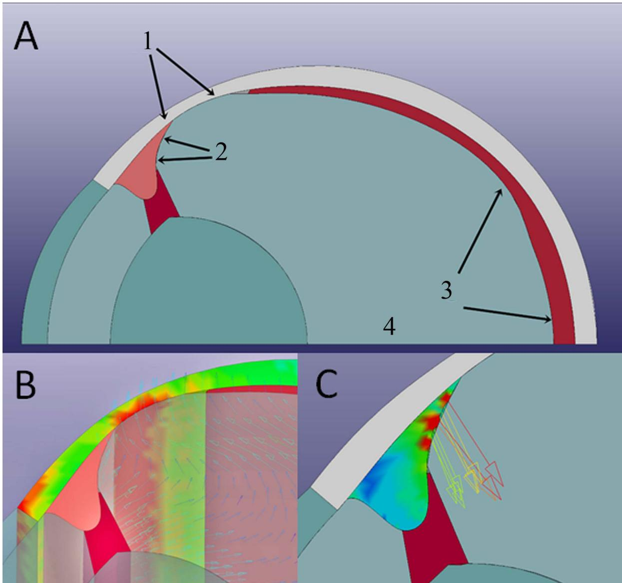
**Figure 6.** (A) Areas of peak stress in sclera (1), ciliary body (2), and retina (3), with location of pressure measurement in the central vitreous (4). (B) Peak stress in sclera at vitreous base (red). Arrows show instantaneous direction of vitreous movement. (C) Peak stress at posterior surface of ciliary body (red). Arrows show instantaneous movement of vitreous attached to ciliary body.
